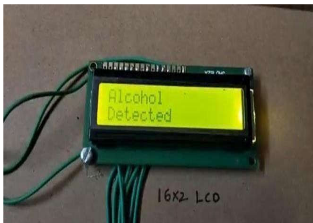
Fig8: LCD Displays Alcohol detected when alcohol is consumed by the driver
