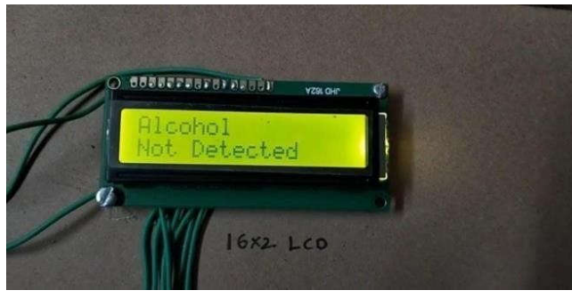
Fig7: LCD Displays Alcohol not detected when alcohol isn't consumed by the driver
