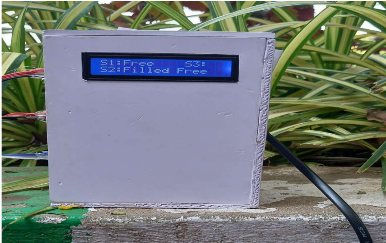
Figure.3. LCD Displaying the information about slot 2 which is Filled
