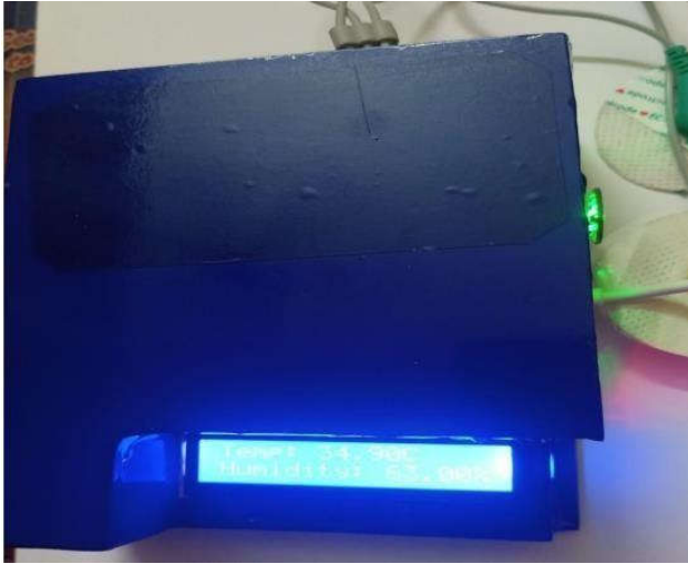
Fig.8. Checking Temperature and Humidity
