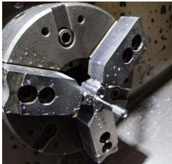
Fig. : Specimen After complete fabrication on one side
