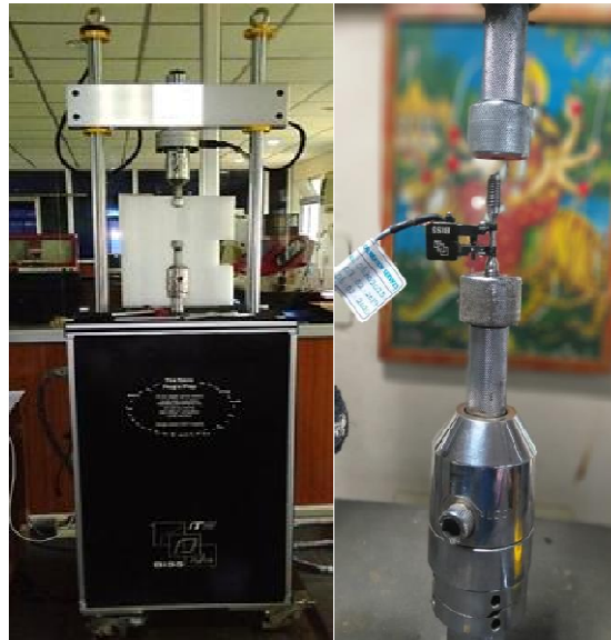
Fig. : Servo Hydraulic Nano UTM (Capacity: 25 KN) used for fatigue testing
