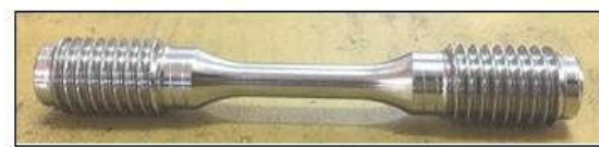
Fig.: Specimen after complete fabrication on both sides without the notch.
