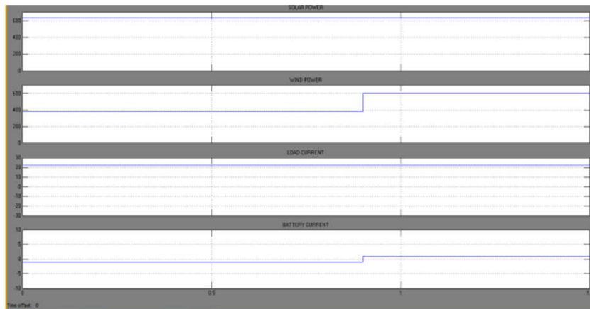
Fig 7: Response of the system during change in Ppv
