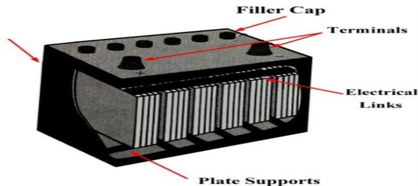
Fig.(3) Lead Acid Battery
