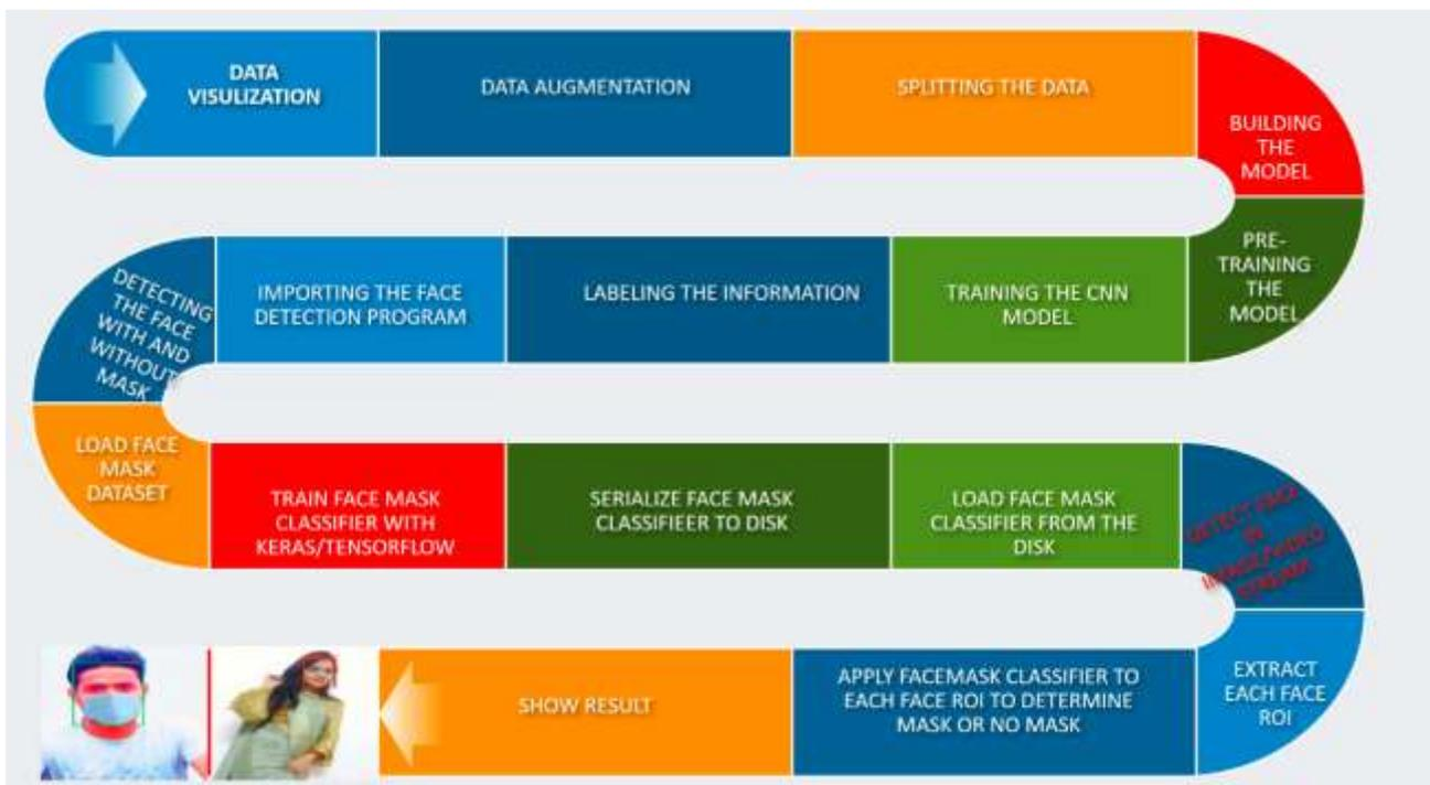
Figure 8: Flow diagram for face mask detection
