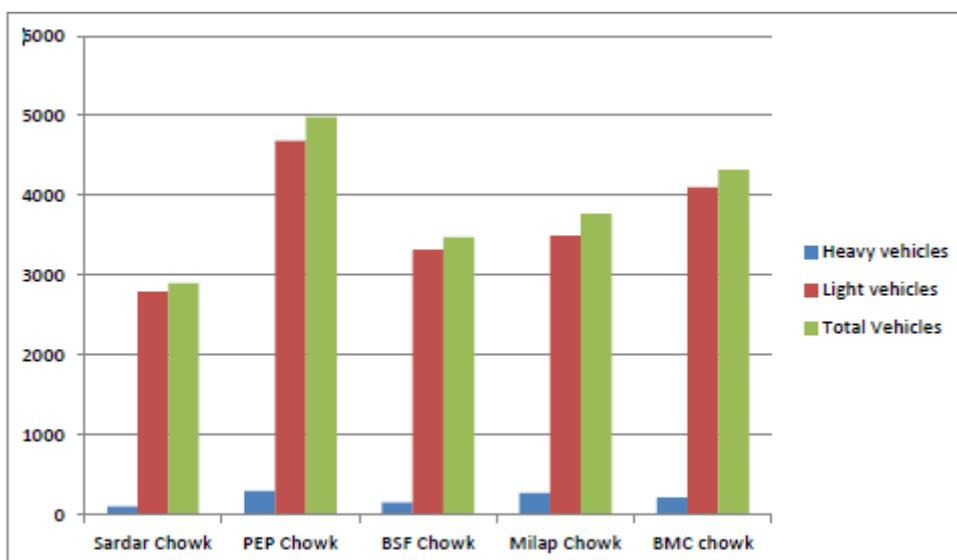
**Figure 3 Maximum Peak Hour Vehicles Volume Distribution on the Intersections**
