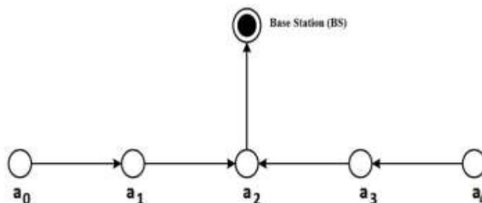
Fig.3.2 Token Passing Scheme in PEGASIS Protocol
