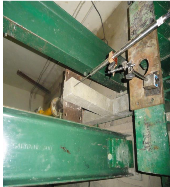
Fig. 8. Testing on Beam-Column joint
