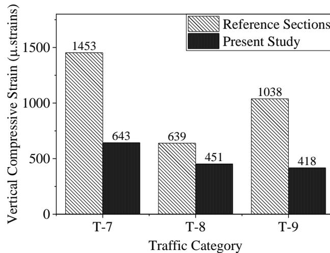
**Figure 2.** The vertical compressive strains on top of the subgrade
