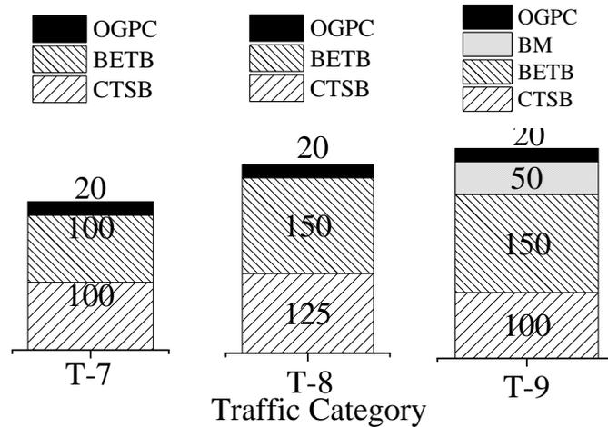
**Figure 3.** Pavement Composition for Bitumen-Emulsion Stabilized Pavements
