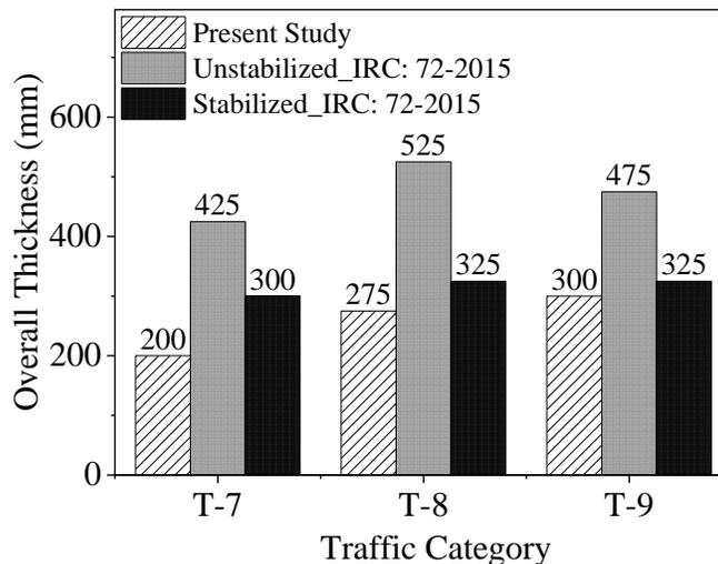
**Figure 4.** Overall thickness Comparison for Bitumen-Emulsion Stabilized Pavements
