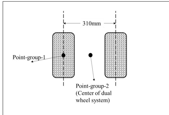
**Figure 1.** Dual Wheel Load System and point groups
