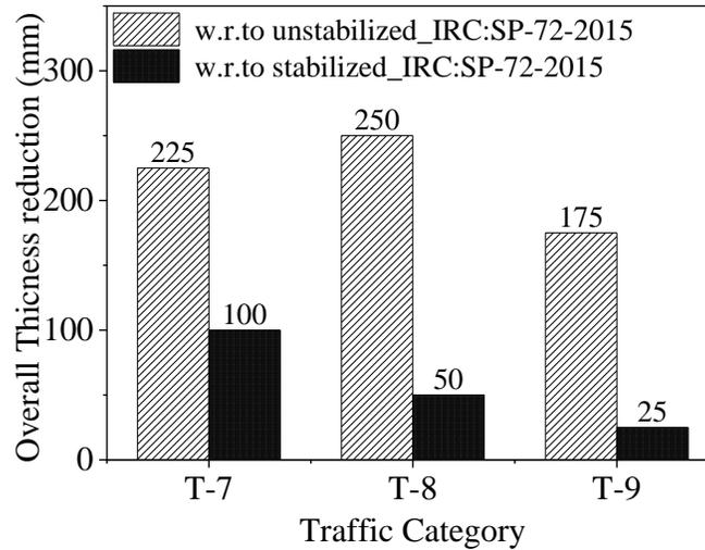
**Figure 5.** Thickness Reduction for Bitumen-Emulsion Stabilized Pavements
