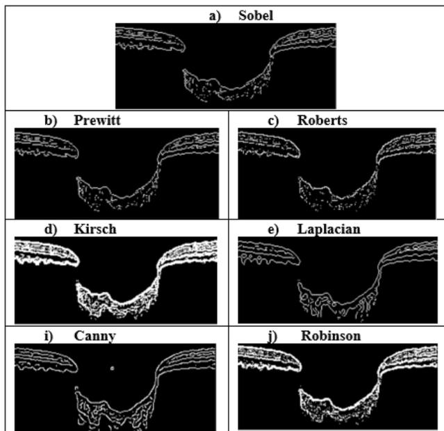
Figure 3. Output of edge-detecting operators
