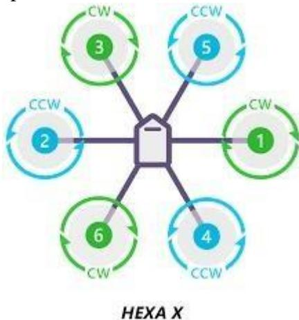
Fig. 1. Frame configuration
