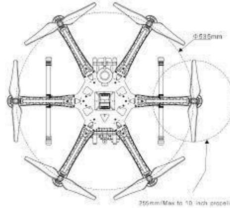
support its operational weight and structural load. Hence, it is necessary to analyze the flexibility and strength of the composing material of the frame. The design of this Fig. 2. Heavy-lift hexacopter frame design
