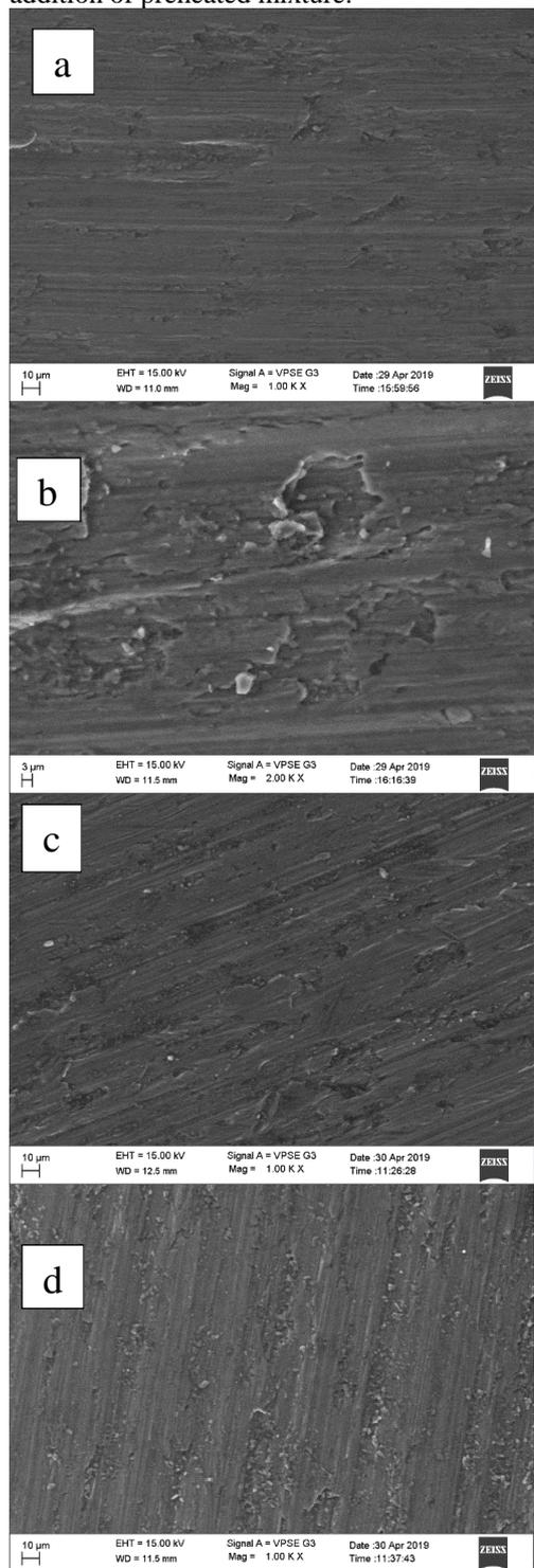
**Fig.3** SEM microphotographs of different composites developed by increasing amounts of Boron Carbide (B<sub>4</sub>C) powder designated as (a) AM (b) AMP2 (c) AMP4 and (d) AMP6
