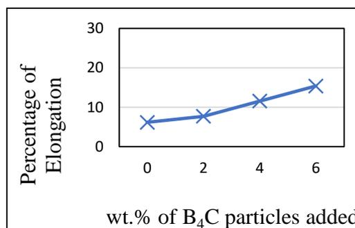
**Fig.8** Percentage elongation variation in Al 6061 alloy and cast composites
