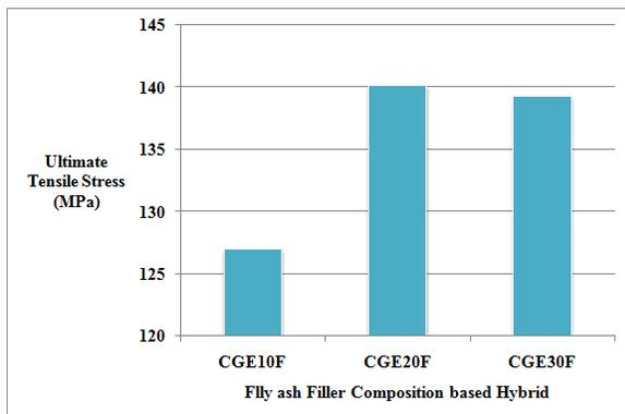
Figure 5. Comparison of ultimate tensile stress of Hybrid Composites
