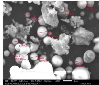
Figure 4. SEM of Fly ash Particles
