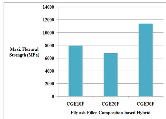
Figure 6. Comparison of Maxi. Flexural Strength of Hybrid Composites
