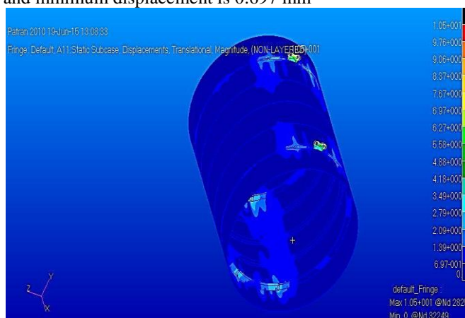
Fig 11: Deformation contour due to wing bending
