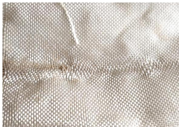
**Fig. 5 Glass fiber membrane**
