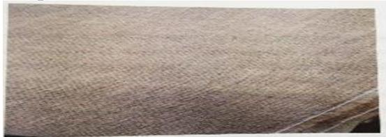
Figure 1. Woven Jute fiber
