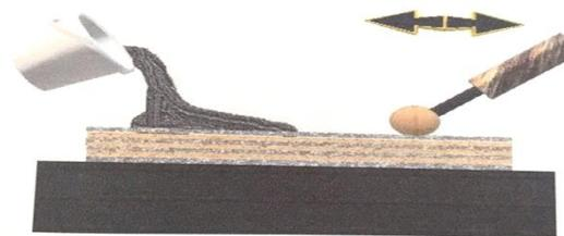
Figure [5]: Hand Lay-Up Process.
