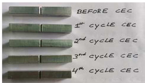
FIGURE 3. Charpy V- Notch impact test specimens after each cycle of CEC process
