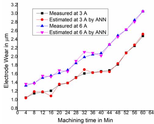
**Fig. 12: Measured and Estimated by ANN for EW of titanium material**
