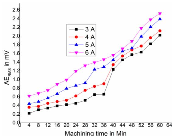
Fig 8:  $AE_{RMS}$  v/s Machining Time for titanium material
