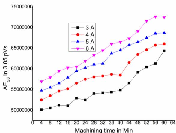
Fig 7:  $AE_{SS}$  v/s Machining Time for stavax material
