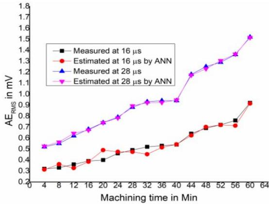
**Fig. 10: Measured and Estimated by ANN for  $AE_{RMS}$  of titanium material**
