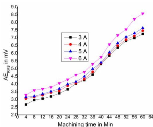
Fig 9:  $AE_{RMS}$  v/s Machining Time for stavax material
