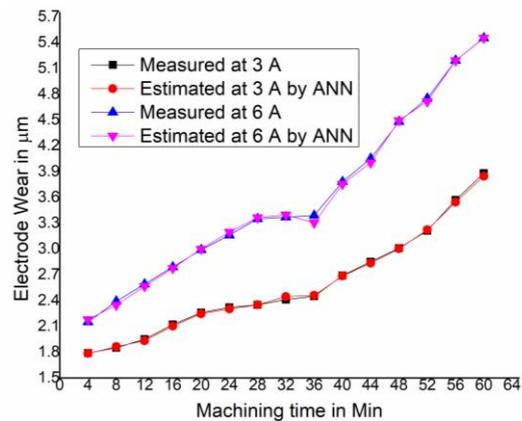
**Fig. 13: Measured and Estimated by ANN for EW of stavax material**
