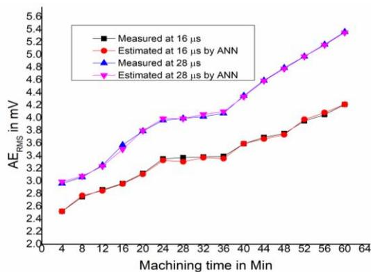
**Fig. 11: Measured and Estimated by ANN for  $AE_{RMS}$  of stavax material**
