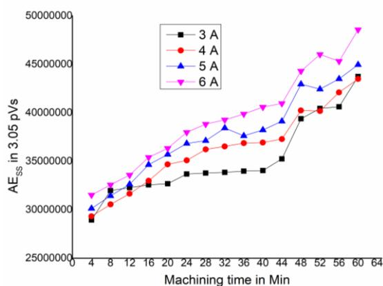
Fig 6:  $AE_{SS}$  v/s Machining Time for titanium material
