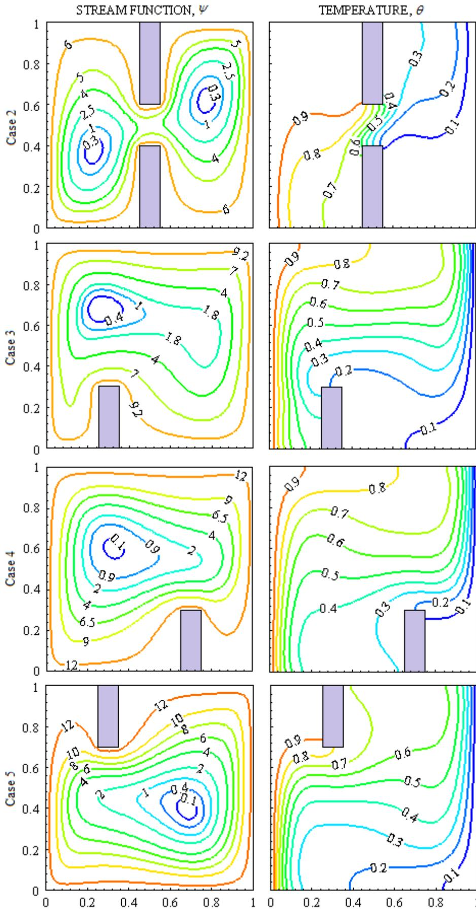
Fig. 4: Contour plots for cases 2 to 5 with Rayleigh number  $Ra = 10^5$ .
