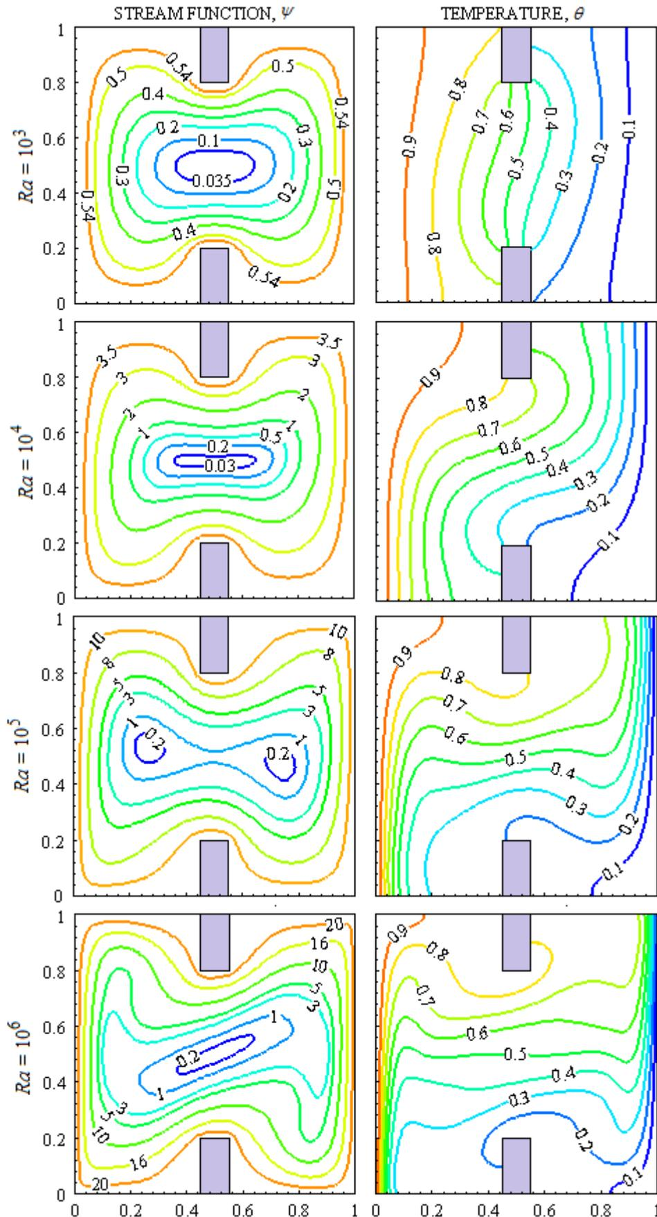
Fig. 3: Contour plots for different Rayleigh number of case 1.
