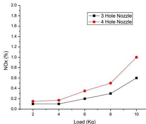
Figure 3.4 Variation of Oxides of Nitrogen vs. Load
