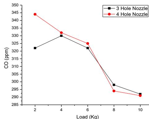
Figure 3.5 Variation of Carbon monoxide vs. Load
