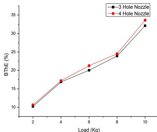
Figure 3.1 Variation of Brake Thermal Efficiency vs. Load
