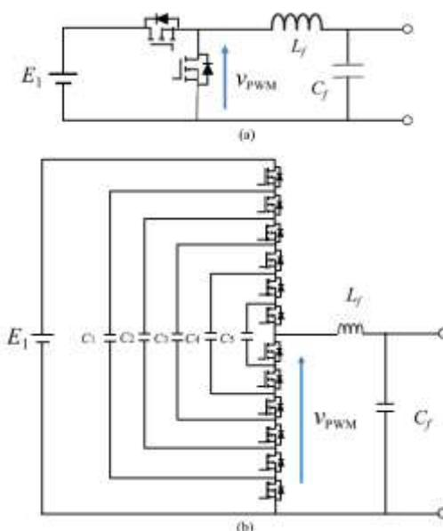
Fig.2: Circuit configurations of power flow controllers. (a) Two-level topology. (b) Multi-level topology (seven-level case).
