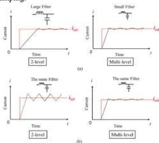
Fig.3: Example of current waveforms in step response depending on the number of output levels and output filter of converters. (a) When both filters are specifically designed for same ripple of output current. (b) When both filters have the same parameters.
