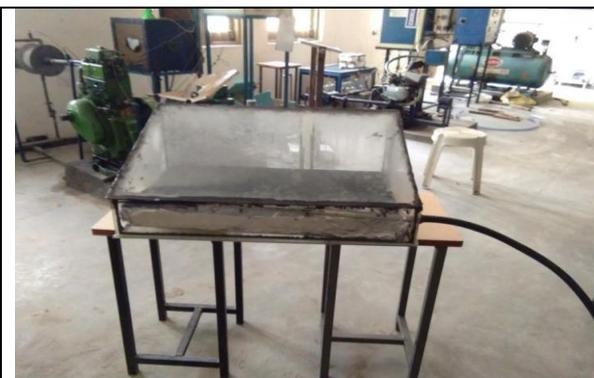
**Figure.5. Fabricated Solar Still With Acrylic Material**
