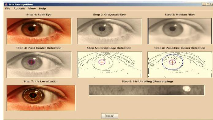
From the above figure we can see an agent will try to load iris images into the database by undergoing all the 8 layers present inside the application. Once it undergo all the intermediate stages ,then it will be passed into a unrolling state. This unrolling image is used as a input to identify the user images which are input during train phase.
