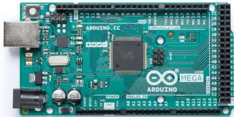
Arduino is one of the main heart of the system. It is one type of microcontroller. The Arduino is used as an ATMEGA 2560P is the microcontroller. And it has 54 digital I/O pins and 16 analog pins, so we can easily use to connect the number of sensors to this development board. The programing and software tool is an open-source platform.
