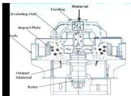
**Figure 3: Vertical Shaft Impactor**
