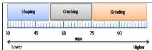
**Figure 4: Effect of rotor velocity on particles in Vertical Shaft Impactor**
