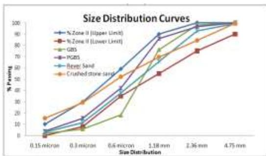
**Figure 6: Size distribution curves of the GBS, PGBS River sand and Crushed stone sand**
