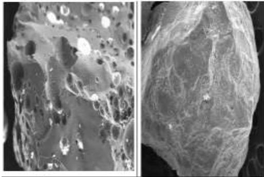
**Figure.1: Comparison of particle morphology (a) River sand (b) GBS**
