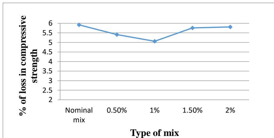
**Figure 1: Compressive strength of concrete specimens for various proportions of the bamboo fiber after 90 days soaking in the chemical water solution.**
