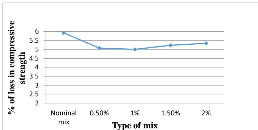
**Figure 2: Compressive strength of concrete specimens for various proportions of the nylon fiber after 90 days soaking in the chemical water solution.**
