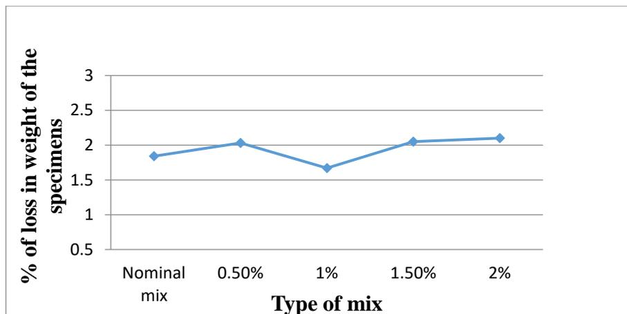
**Figure 3: Results of sulphate attack on concrete specimens for various proportions of the bamboo fiber after 90 days soaking in the chemical water solution.**
