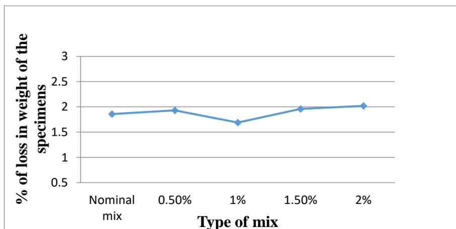
**Figure 4: Results of sulphate attack on concrete specimens for various proportions of the nylon fiber after 90 days soaking in the chemical water solution.**
