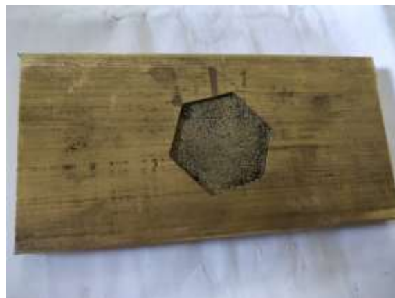
Figure 6: Brass metal after machining
