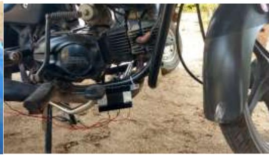
Fig.9 TEG mounted on the silencer
