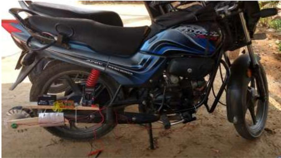
Fig.7 Turbine and TEG mounted on the vehicle
