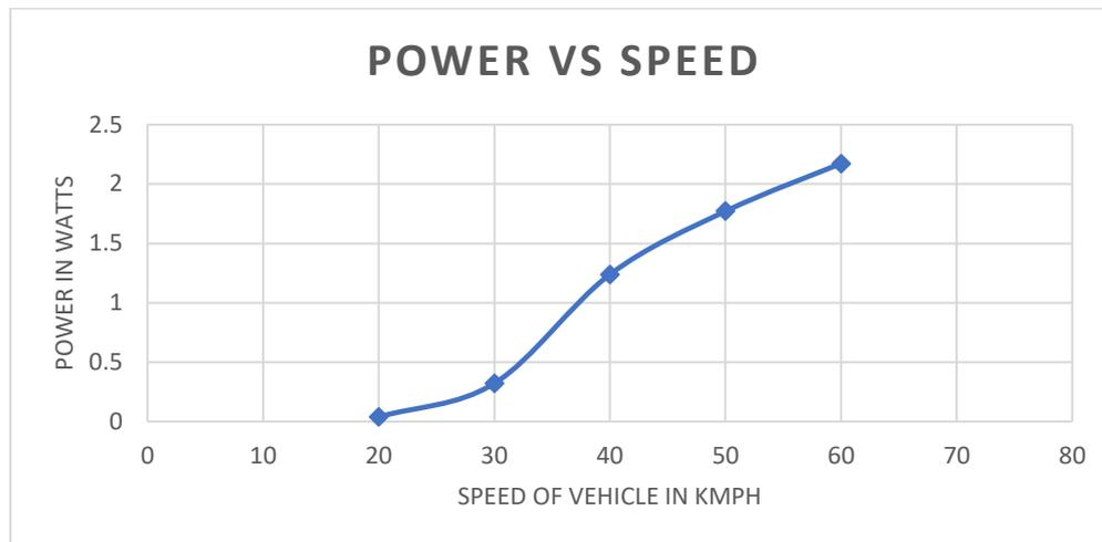
Fig.17 Graph of speed of vehicle vs Power output
