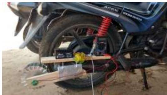
Fig.15 Turbine mounted on the bike
