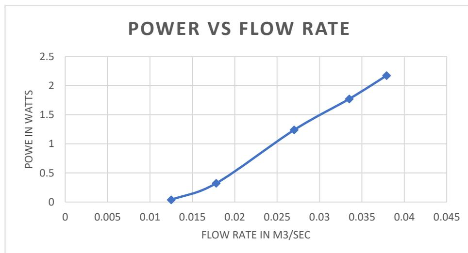
Fig.16 Graph of flow rate of exhaust gas vs power output
