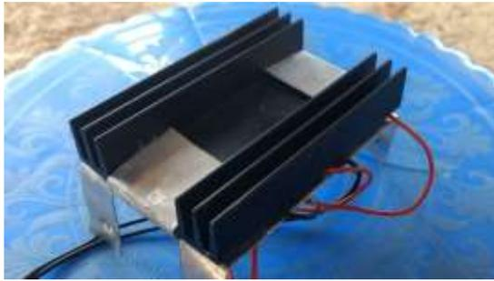
Fig.8 TEG module with alluminium fin
