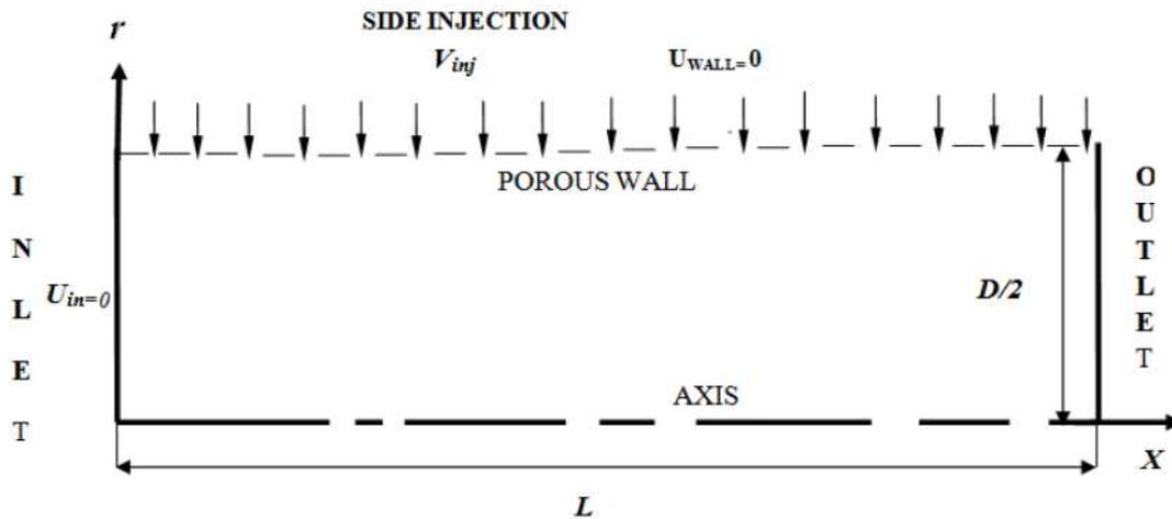
Figure 1, Schematic diagram for the circular axi-symmetric conduction by porous wall and closed inlet with lateral injection..
