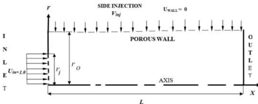
Figure 2, Schematic diagram of the axially symmetrical circular conduit with porous and partially opened inlet for side injections
