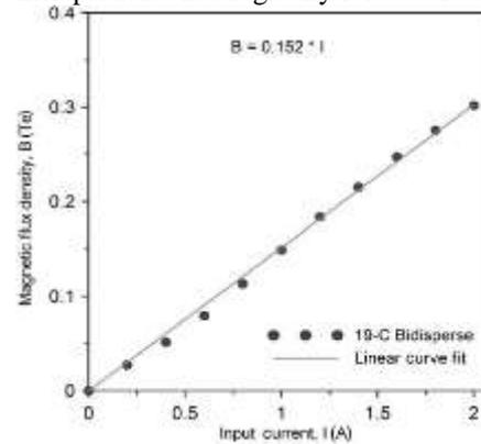
Figure 2. The magnet flux density adjustment (B, T) depending on the input current at the distance between the viscometer 's parallel discs.
