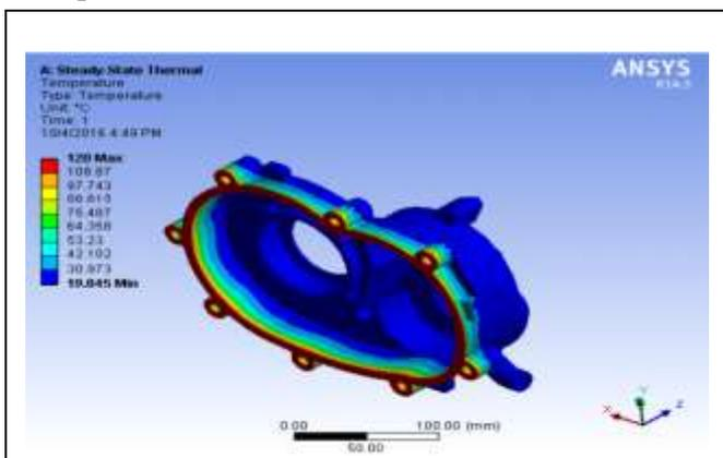
Fig 28. Temperature of Aluminum alloy
