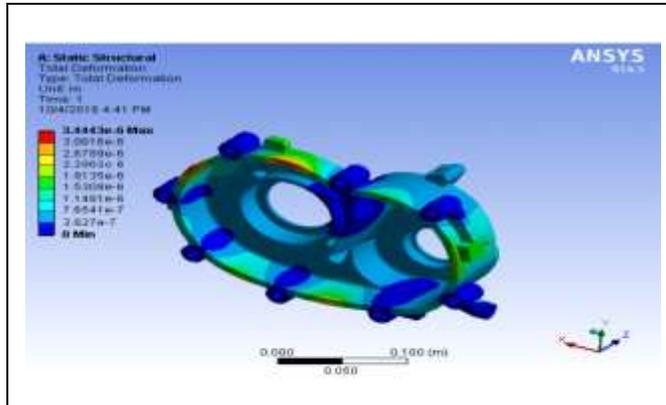
Fig.13. Deformation of Steel
