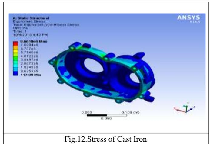
Fig.12. Stress of Cast Iron
