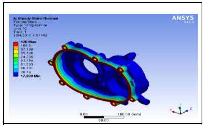
Fig 24. Temperature of Cast Iron
