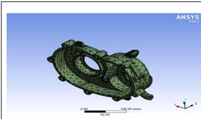
Fig 27. Meshed model of Aluminum alloy
