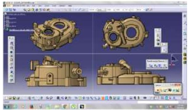
Fig.4. All views if gear box casing
