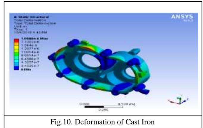
Fig.10. Deformation of Cast Iron
