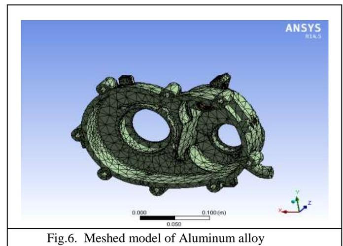
Fig.6. Meshed model of Aluminum alloy
