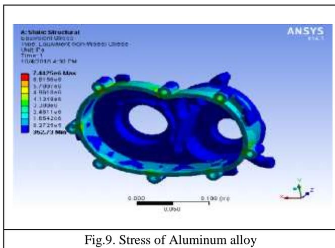
Fig.9. Stress of Aluminum alloy
