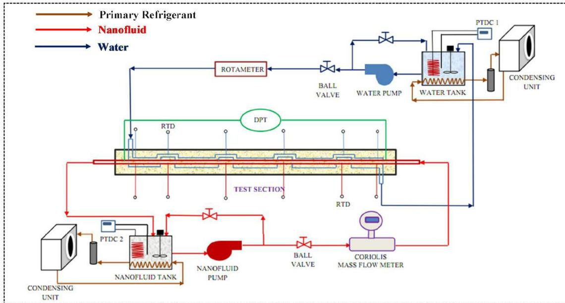
**Figure 2:** schematic of the experimental apparatus
