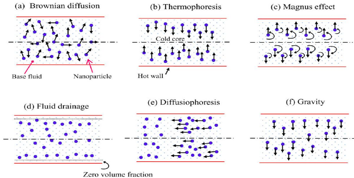
**Figure 1. Graphical representation of slip mechanisms**
