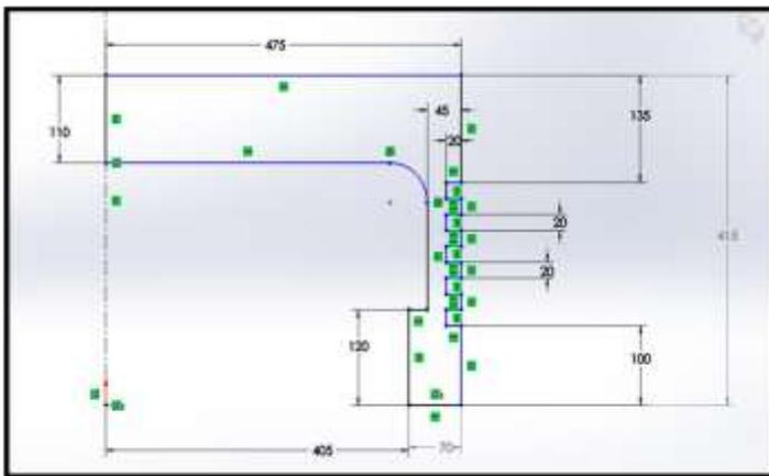
Fig 1: Sketch Dimensions of piston
