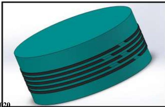
Fig 5: Complete Assembly of Piston and piston rings
