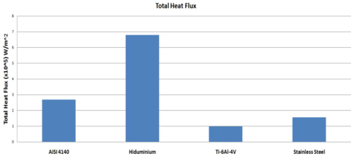
**Fig 25: Comparison of all materials in Total Heat Flux**
