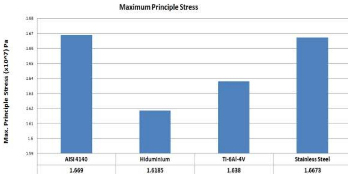
Fig 15: Comparison of all materials in Maximum Principle Stress
