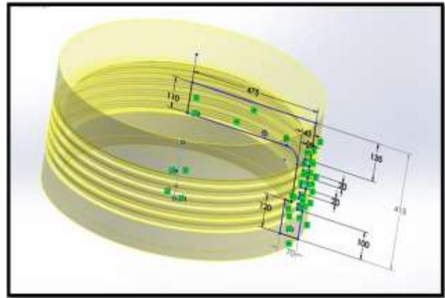
Fig 2: Revolved Base of piston
