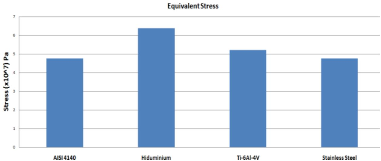
Fig 14: Comparison of all materials in Equivalent Stress
