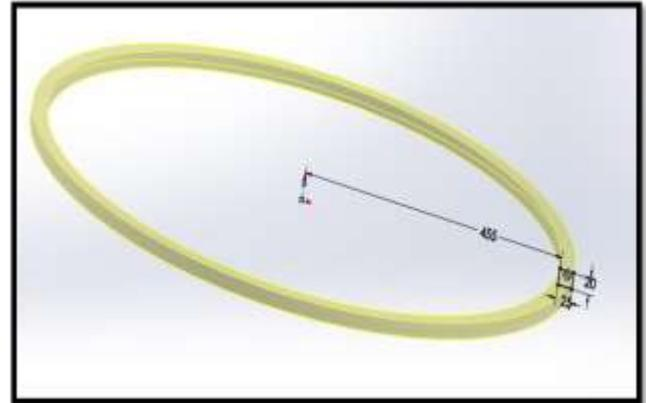
Fig 4: Revolved base of piston ring
