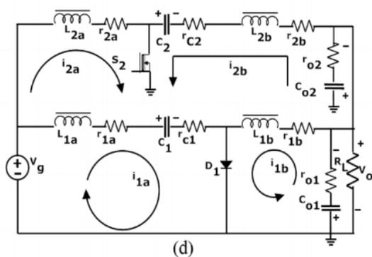
Circuit diagram of interleaved cuk converter with different modes of operation.(a)basic circuit (b)S1 ON and S2 OFF (c)S1 and S2 OFF(d) S1 OFF and S2 ON
