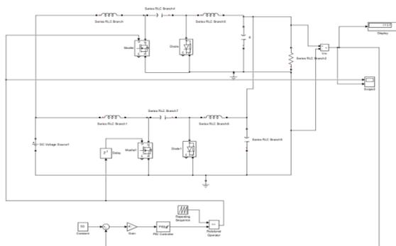
Fig2: PID controlled interleaved cuk converter
