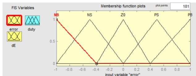
Fig3 Membership function plot for input 'error'
