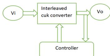
Above figure shows the basic block diagram of the closed loop interleaved cuk converter. Output voltage is first sent to the controller ( PI, PID or FLC) and compared with the reference or set voltage. Resultant error signal is then used to compensate the duty signal of the switch and the process continuous till the set value is reached.
