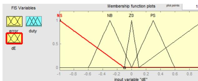
Fig4: Membership function plot for input 'dE'
