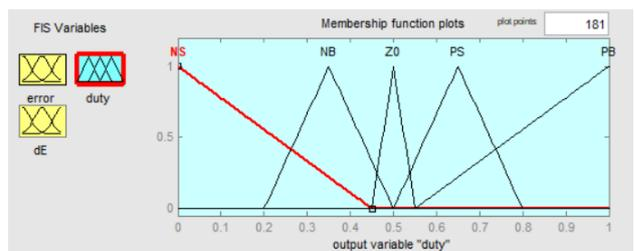
Fig5: Membership function plot for output 'duty'
