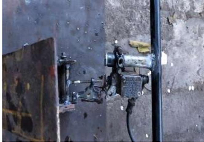
FIG 4.3: SINGLE PEDAL WITH MASTER CYLINDER
