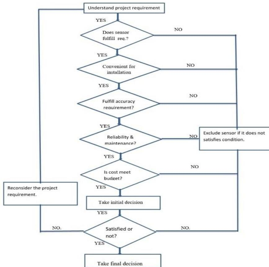
Figure(2): Procedure for the selection of sensor technology.
