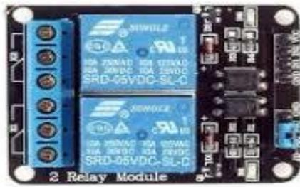
Fig 5: 2 Channel Relay
