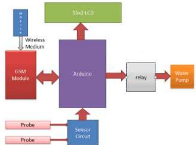
Fig.1. Block diagram of automatic irrigation system
