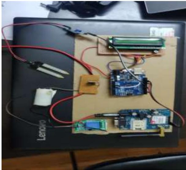
Fig 2 Hardware implementation of automatic irrigation system using Arduinouno
