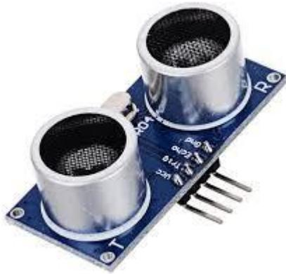
Figure 3: Ultrasonic sensor
