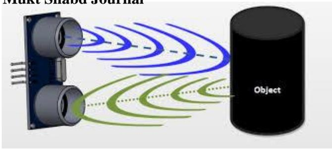
Figure 2: Working of ultrasonic sensor
