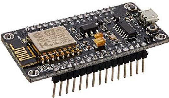
Figure 4: ESP8266 Microcontroller
