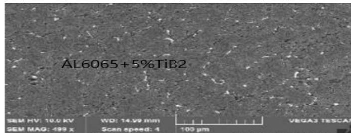
**Figure: Micro structure of Al6061 and 5% of TiB<sub>2</sub>**
