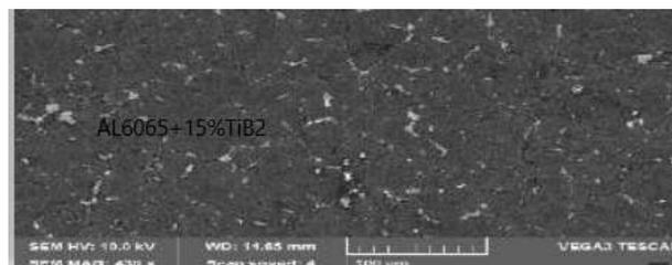
**Figure: Micro structure of Al6061 and 15% of TiB<sub>2</sub>**
