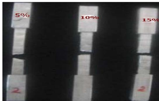
**Figure: Tensile Specimens after test**
