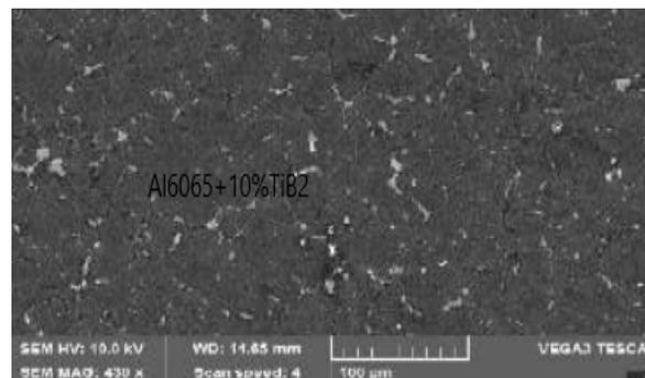
**Figure: Micro structure of Al6061 and 10% of TiB<sub>2</sub>**
