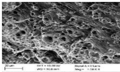
**Figure: SEM image of ultimate tensile strength sample Al6061 and 15% of TiB<sub>2</sub>**
