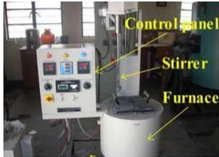
**Figure: Stir Casting Setup**
