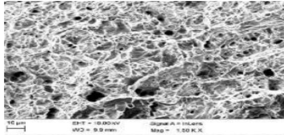
**Figure: SEM image of ultimate tensile strength sample Al6061 and 5% of TiB<sub>2</sub>**
