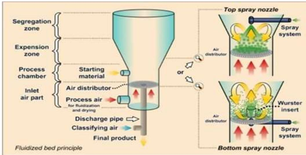
**Fig 1: Air suspension method**
