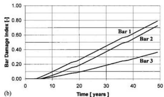
fig 6: damage index of time history analysis (I)graph showing three different concrete cells (II) graph showing three different steel bars.
