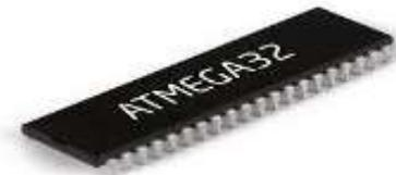
ATmega32 is an 8-bit AVR microcontroller that takes input from flex sensors and then computes the output by using the algorithm which is stored inside the microcontroller.
