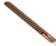
Flex sensors that are mounted on the glove are used to measure the amount of bending made by our Hand while wearing the glove consisting of the flex sensors. Usually, flex sensors are used to measure the resistance incurred at a different angles of the flex sensors.
