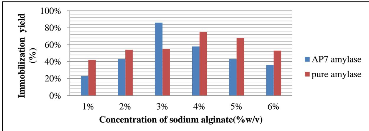
Figure 4: Effect on immobilization yield of  $\alpha$ -amylase with various sodium alginate concentrations
