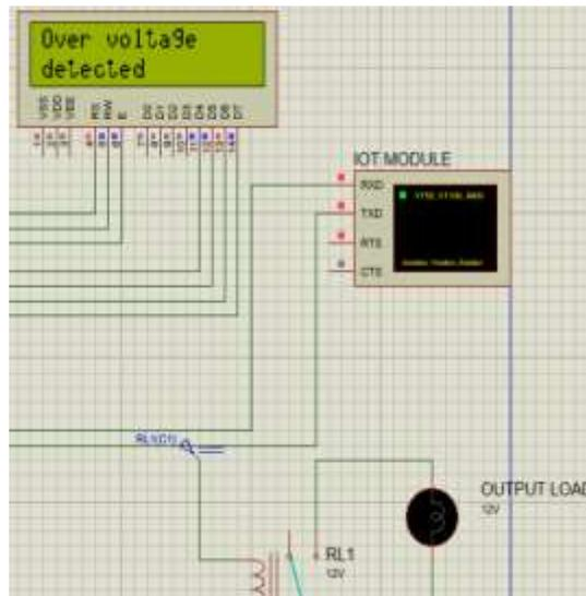
Figure 4: After the execution, over voltage is detected when the voltage value is reached beyond its threshold value and load is tripped off
