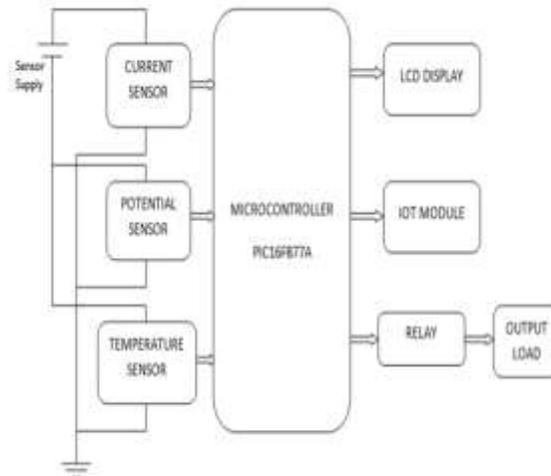
Figure 1: Software Simulation block diagram of proposed system
