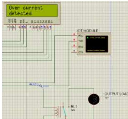
Figure 3: After the execution, over current is detected when the current value is reached beyond its threshold value and load is tripped off.
