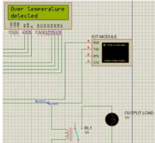
Figure 5: After the execution, over temperature is detected when the temperature is reached beyond its threshold value and load is tripped off.
