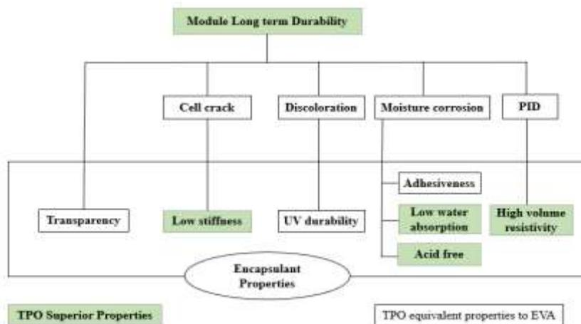
Fig. 1 Properties of TPO & EVA encapsulant materials
