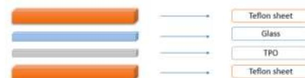
Fig. 3 Lamination Structure of TPO encapsulant for UV-Visible spectroscopy
