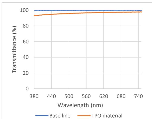
Fig. 5 (a) Transmittance of TPO sample in visible range
