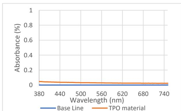
Fig. 5 (b) Absorbance of TPO sample in visible range
