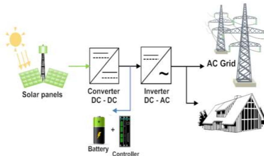
Fig. 6 General structure of PV energy.
