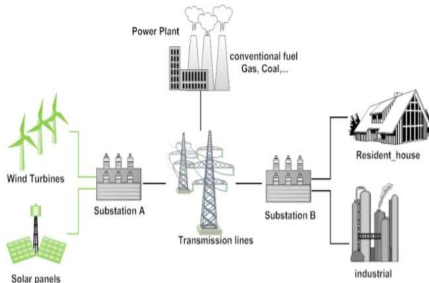
Fig. 3 The general structure of integrating renewable energy into AC Grid
