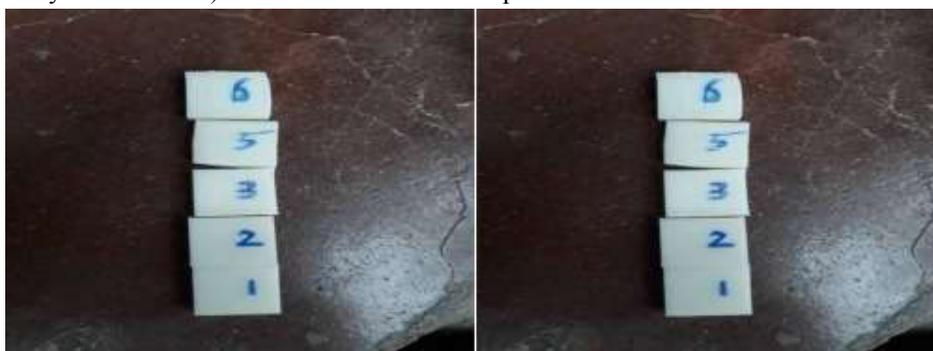
FIGURE 11.3 Before and After Testing of Shore Hardness Test Specimen
